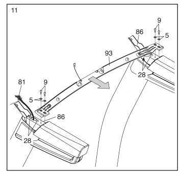
12. With the help of a second person, hold the console assembly near the left Handrail (86) and the right Handrail (not shown).
